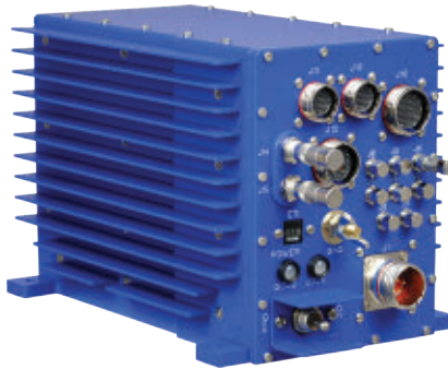
This ATR chassis is an example of the high amount of I/O that one box had to accommodate. The unit is about the size of a half-ATR box.
