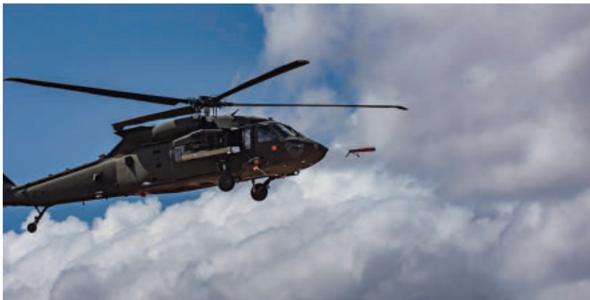
An Area-I Air-Launched, Tube-Integrated, Unmanned System, or ALTIUS, is launched from a UH-60 Black Hawk at Yuma Proving Ground, Ariz., where the Army led a demonstration that highlighted the forward air launch of the ALTIUS.
