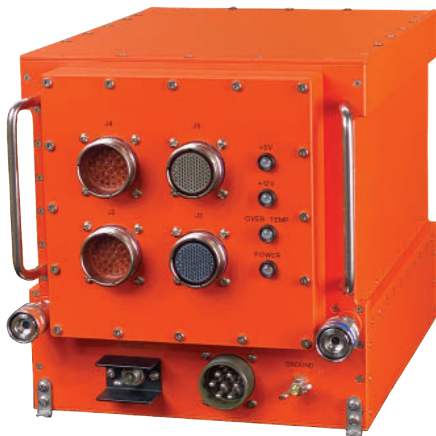
The Elma VITA 48.4 liquid flow-through ATR box with a 6U Open-VPX backplane can accommodate as many as eight boards and two VITA 62 plug-in power supplies
