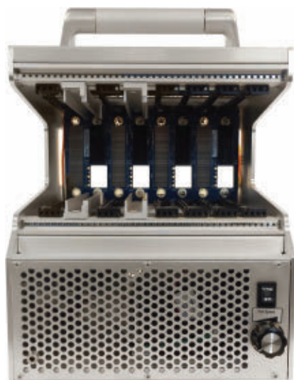
The Pixus open frame development chassis for OpenVPX/SOSA applications features four VPX power and ground-only slots, four VITA 67.3c cutouts, and SOSA clocking.
